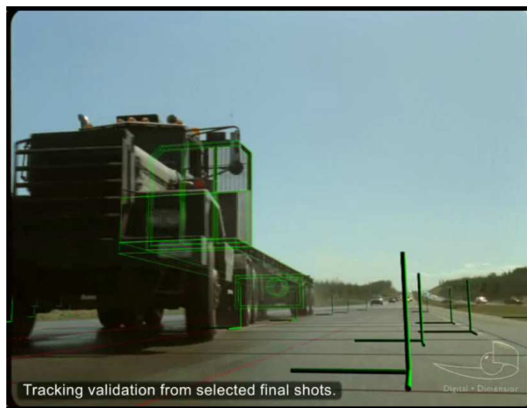
Figure 5.2: The verification of the camera matching with simple 3D objects inserted into the live action footage. (Digital Dimension Studio, ©New Line Cinema)
