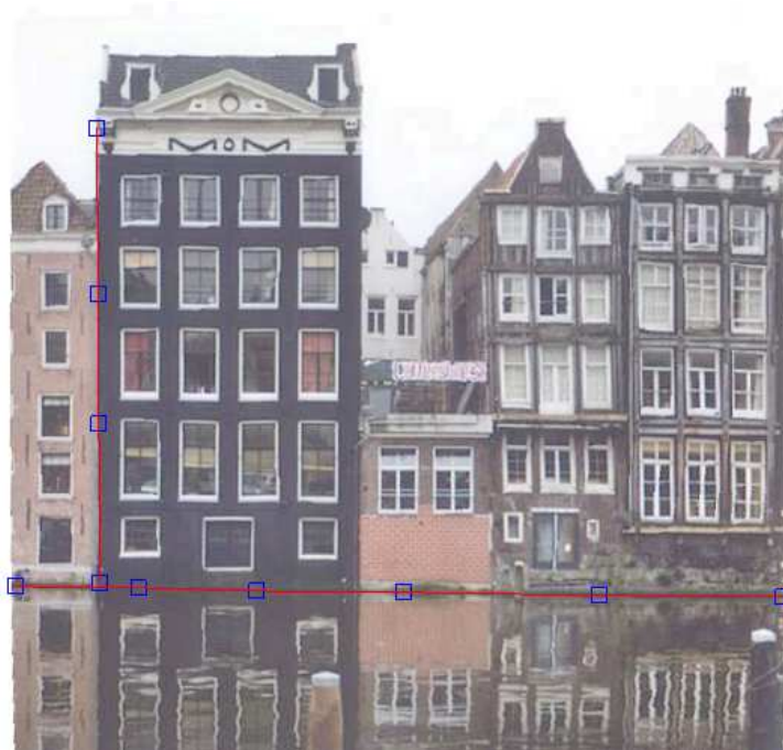
Figure 3.7: The parameters are automatically calibrated and the lines become straight.
